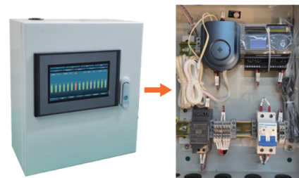
Pre-install & pre-wiring for BMS, BMS600Pro and HMI-Gate (optional)
